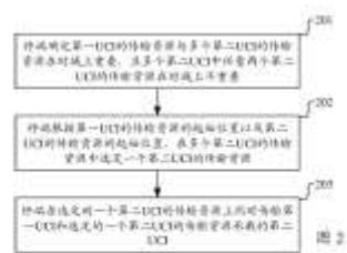
201: A terminal determines that a transmission resource of a first UCI overlaps transmission resources of a plurality of second UCIs in a time domain, and the terminal determines the initial position of the transmission resource of the first UCI and the initial positions of the transmission resources of the second UCIs. 202: The terminal selects one second UCI from the second UCIs according to the initial position of the transmission resource of the first UCI and the initial positions of the transmission resources of the second UCIs. 203: The terminal simultaneously transmits the first UCI and the selected second UCI on the transmission resource of the selected second UCI.
